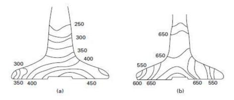
**Figure 4.5:** Temperature distribution (°C) of valves during operation. An air-cooled 200 cm<sup>3</sup> engine. (a) Inlet valve (30  $\phi$ mm). (b) Exhaust valve (26  $\phi$ mm).
