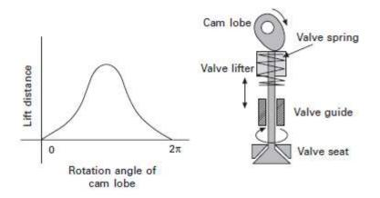
**Figure 4.3:** Rough sketch of a valve train showing valve lift distance in the valve timing diagram. The lift distance (vertical arrow) given by the cam lobe is the displacement along the axial direction of the valve.
