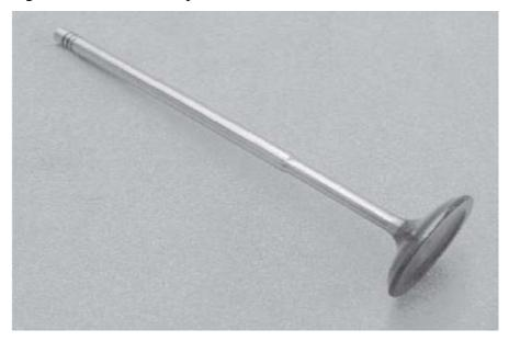
**Figure 4.1:** Exhaust valve. The inlet valve has a similar shape, but the crown size is normally larger than that of the exhaust valve.
