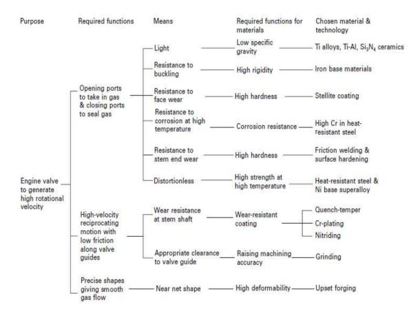
Figure 4.4: Functions of valves
