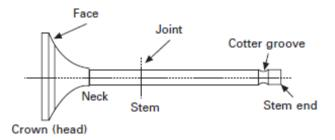
Figure 4.2: Nomenclatures of the valve. The shape from the crown to the neck is designed to give a smooth gas flow.
